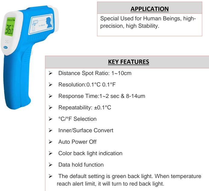
Alarm function: The alert limit of the alarm function is 37.5°C as default. When the reading reaches 37.5°C, the buzzer will ring with" Bi, Bi, Bi" sound and the back light will turn red.
